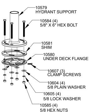
**SRH-MS Complete Roof Hydrant & Mounting System** Shipped in Cartons 1 & 2
