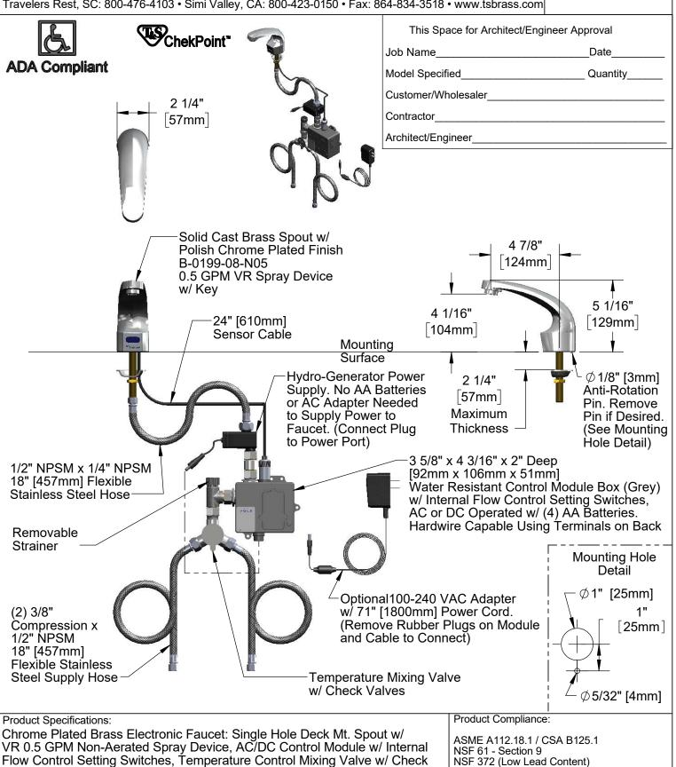
Valves, Hydro-Generator, 18" Flexible Stainless Steel Supply Hoses
