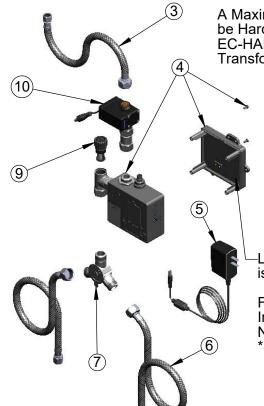
A Maximum of (8) ChekPoint Faucets can be Hardwire Connected and Powered by EC-HARDWIRE ChekPoint Hardwire AC Transformer. (Sold Separately)
