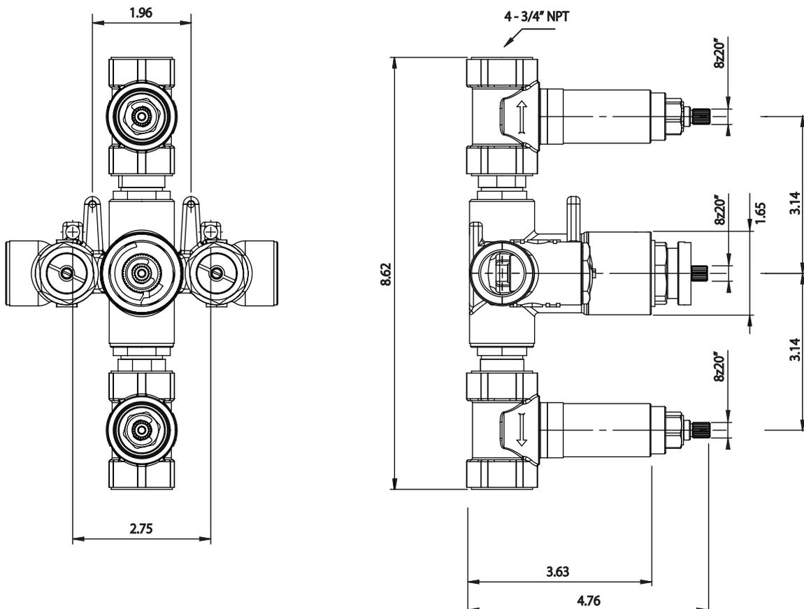
TVH.4401 | 3/4" Thermostatic Valve With 2 Independent Volume Controls Page 2 of 2
