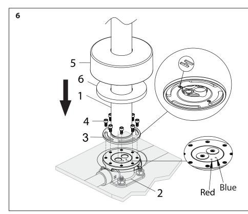
Insert trim (1) onto the valve (2). Secure the trim (1) to the valve (2) using screws (4). Tighten screws with wrench provided. Then push round cover (5) and washer (6) to the base.
