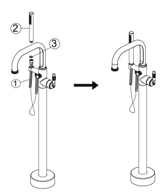
Connect the shower hose (1) to the hand held (2). Ensure that the washer (3) is inserted into the end of the shower hose (1).
