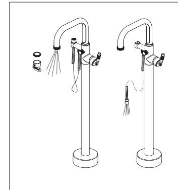
After Installationis complete remove the aerator with the provided aerator key and flush the water lines. Turn on the hot and cold supply lines and allow water to flow for approximately 1 minute. After flushing re-insert the aerator.
