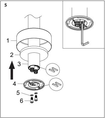
Before installing the trim ensure double o-rings are undamaged and greased. Please the round cover (1) and washer (2) over the stand pipe (3). Install the round connector (4) to the faucet body using the washer (5) and screws (6) with Allen wrench provided. Do not over tighten.
