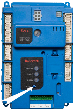
Figure 28. Reset Button on Controller
